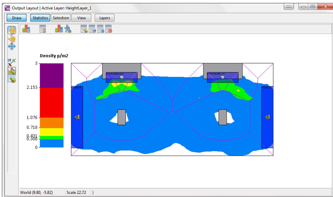
Figure 16: The 2D output window showing the density map.
