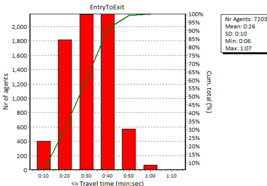
Figure 9: Walking time histogram showing all pedestrian movements between any Entry activity (either Entrance or Platform) to any Exit activity (also either Entrance or Platform). The bar at indicates the agents that took <10s. The second bar indicates the agents that took 10 to 20s, etc.
