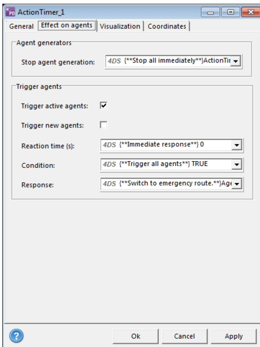
Figure 10: The Effect on agent page of the Action timer. After the Incident stop the generation of all agents and reroute the agents to the Emergency\_route.
