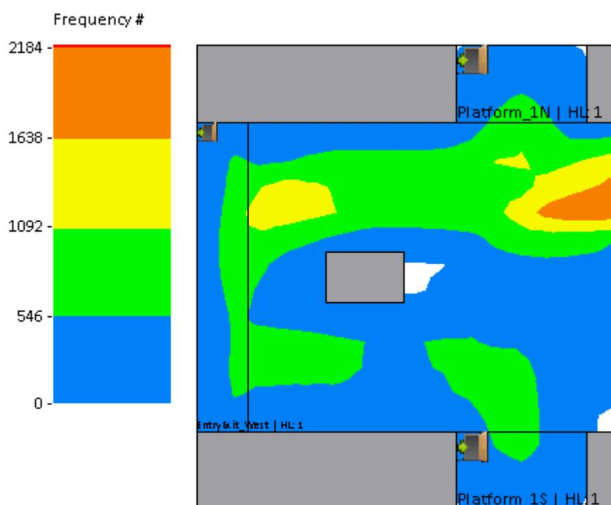
Figure 4: Frequency map of the West side of the station with colors indicating the absolute number of pedestrians passing there.
