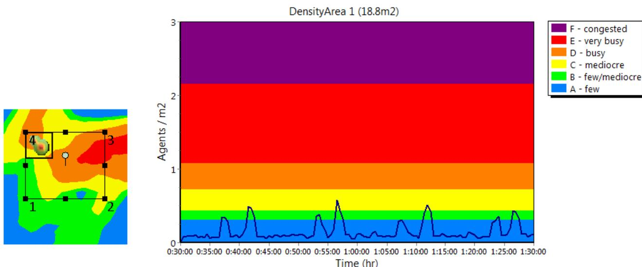
Figure 8: Area Density graph. The horizontal axis shows time. The vertical axis shows the crowd density in Persons per square meter.
