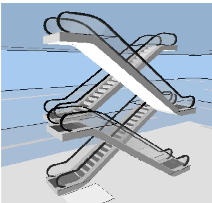
Figure 14: Criss Cross configuration of escalators.
