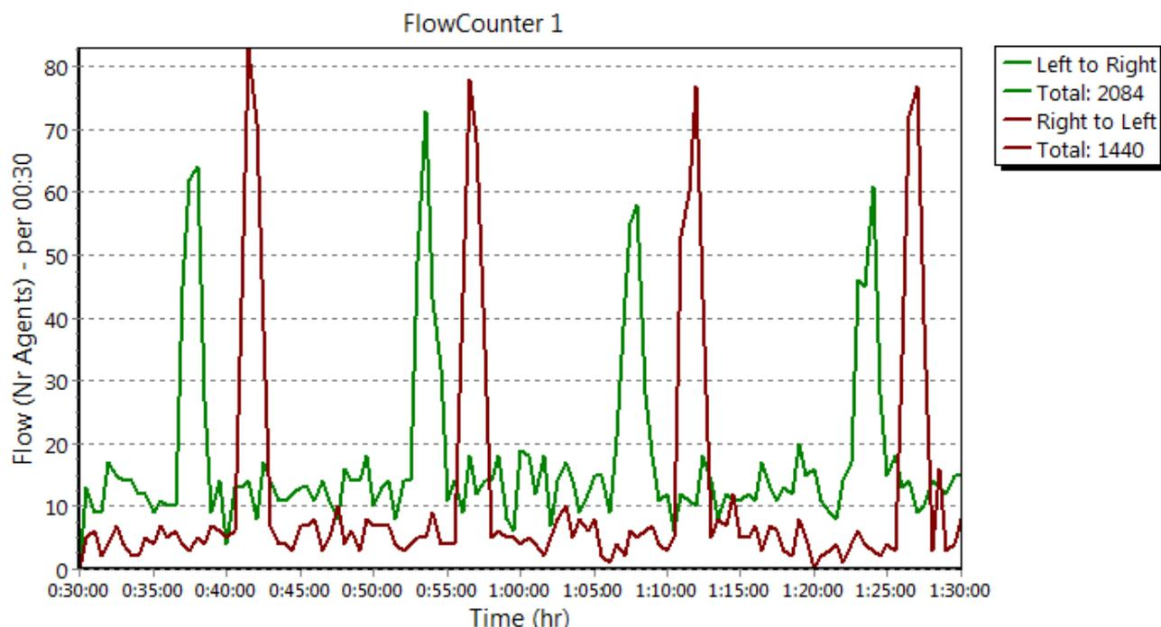
Figure 7: Flow counter graph obtained by clicking a flow counter line. The horizontal axis shows time. The vertical axis displays the flow in Agents per time unit, where the time unit, typically 30 seconds, is configured in the Output Settings.
