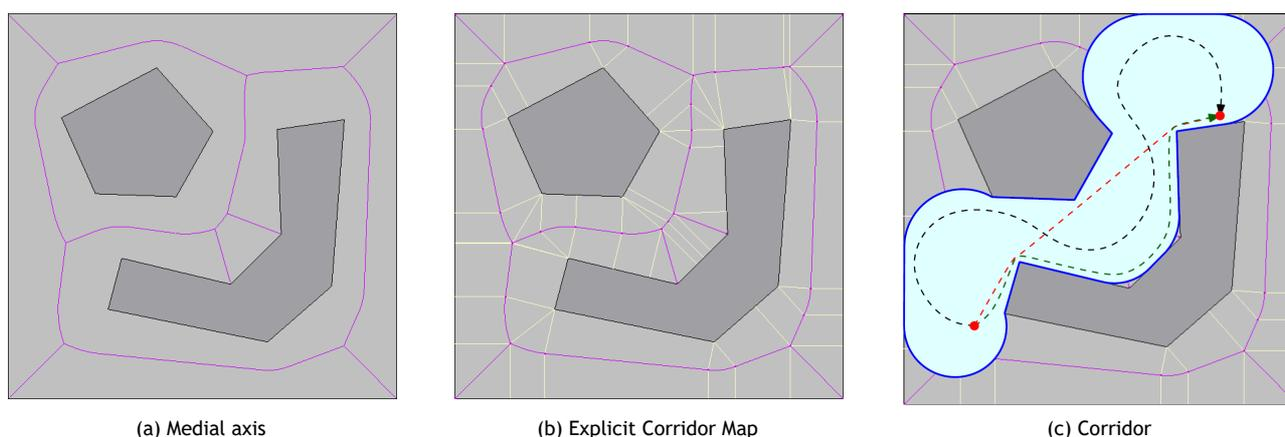
Figure 1: (a) The medial axis, shown in purple, runs through the middle of the walkable space. (b) Closest-point annotations, shown in yellow, turn the medial axis into the ECM navigation mesh. (c) The corridor, shown in blue. The dotted lines show several possible routes through the corridor from the start position to the goal.
