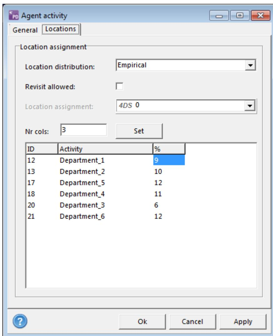
Figure 6: The Locations settings of the Shop activity. Note that the percentages of the Empirical distribution do not add up to 100% the remaining fraction gives the probability that the agent will skip this activity.
