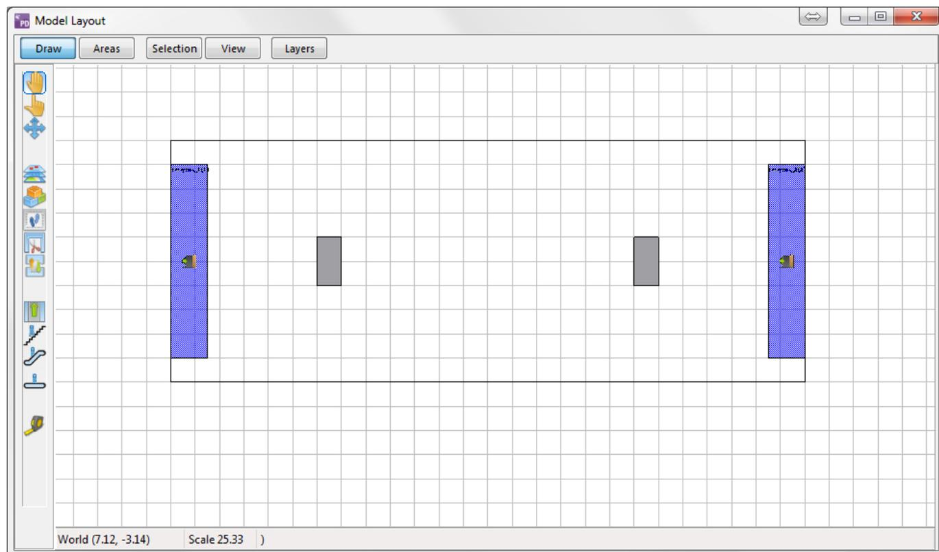
Figure 3: We are now ready to run our pedestrian flow model for the first time. With the default settings, pedestrians will enter through either of the Entry/Exit areas and leave the model through the other.
