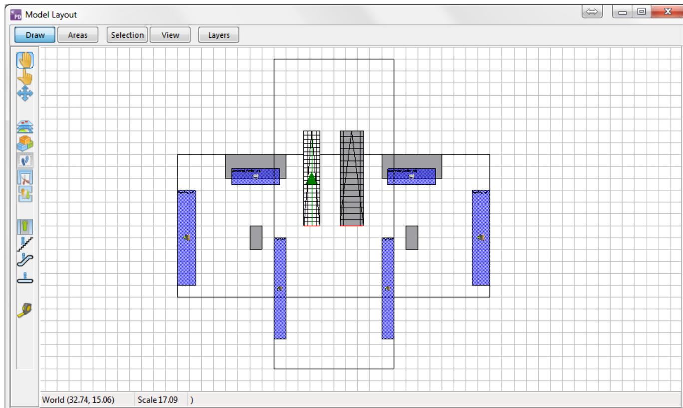
Figure 24: The Model Layout window with the two Height layers an escalator and a flight of stairs form a connection between the two layers.
