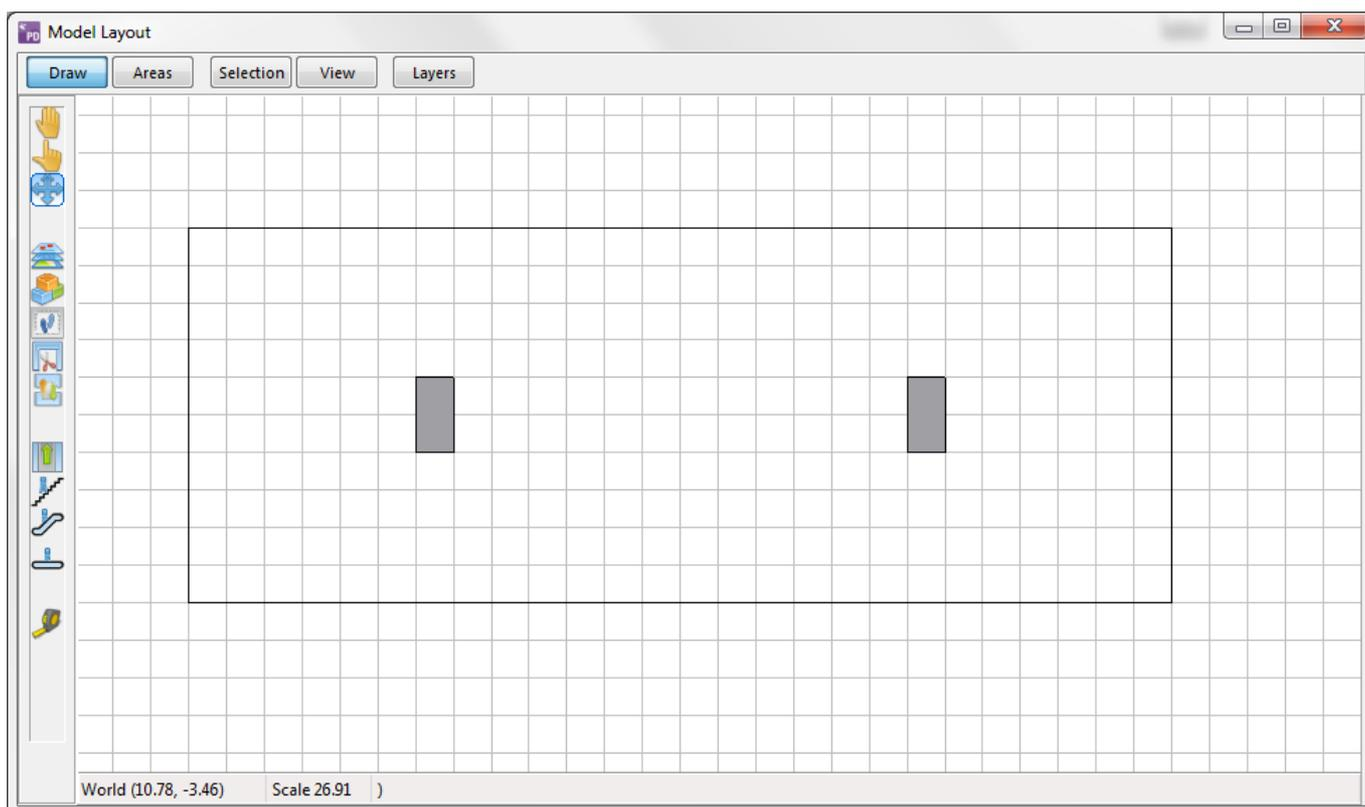
Figure 2: The Model Layout window showing the tunnel with the two Obstacles that represent the concrete columns that support the tracks.
