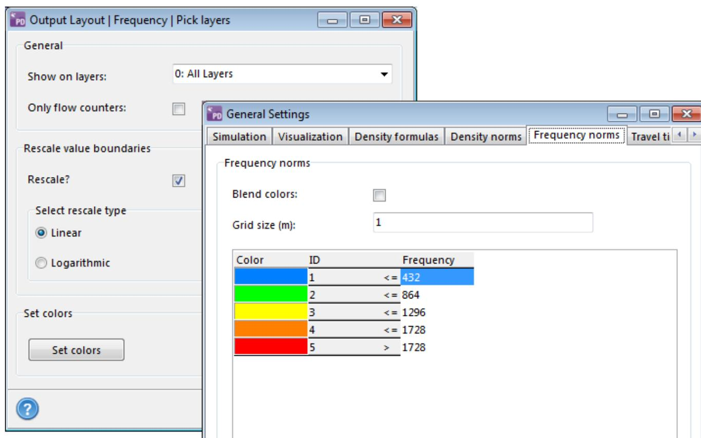
Figure 5: The frequency map dialog. If Rescale is enabled, colors are chosen automatically, either according to a linear or logarithmic scale. If it is disabled, the colors can be configured manually.
