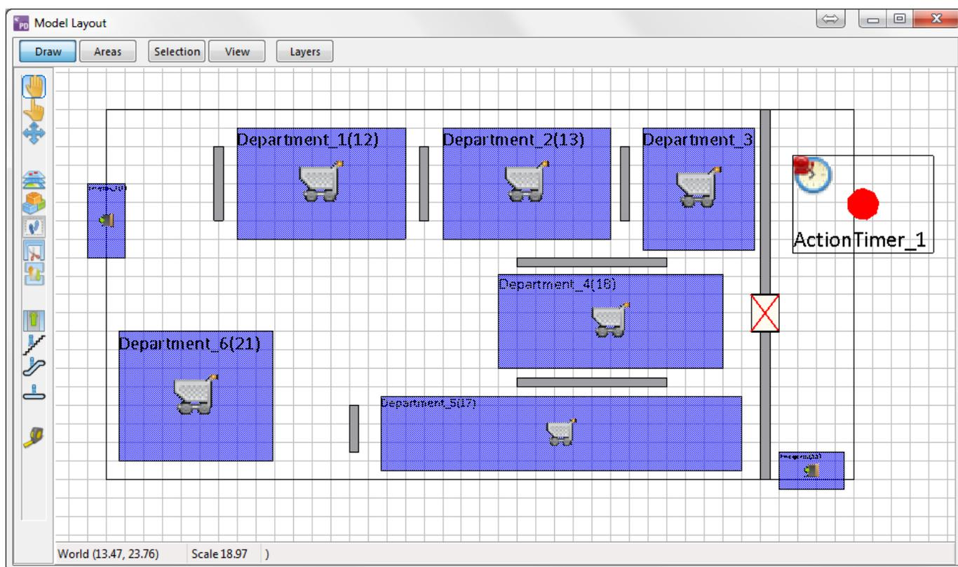
Figure 12: The Model Layout with the ground floor of the department store with an Action timer. The Passageway used as an emergency exit is closed before the incident occurs.
