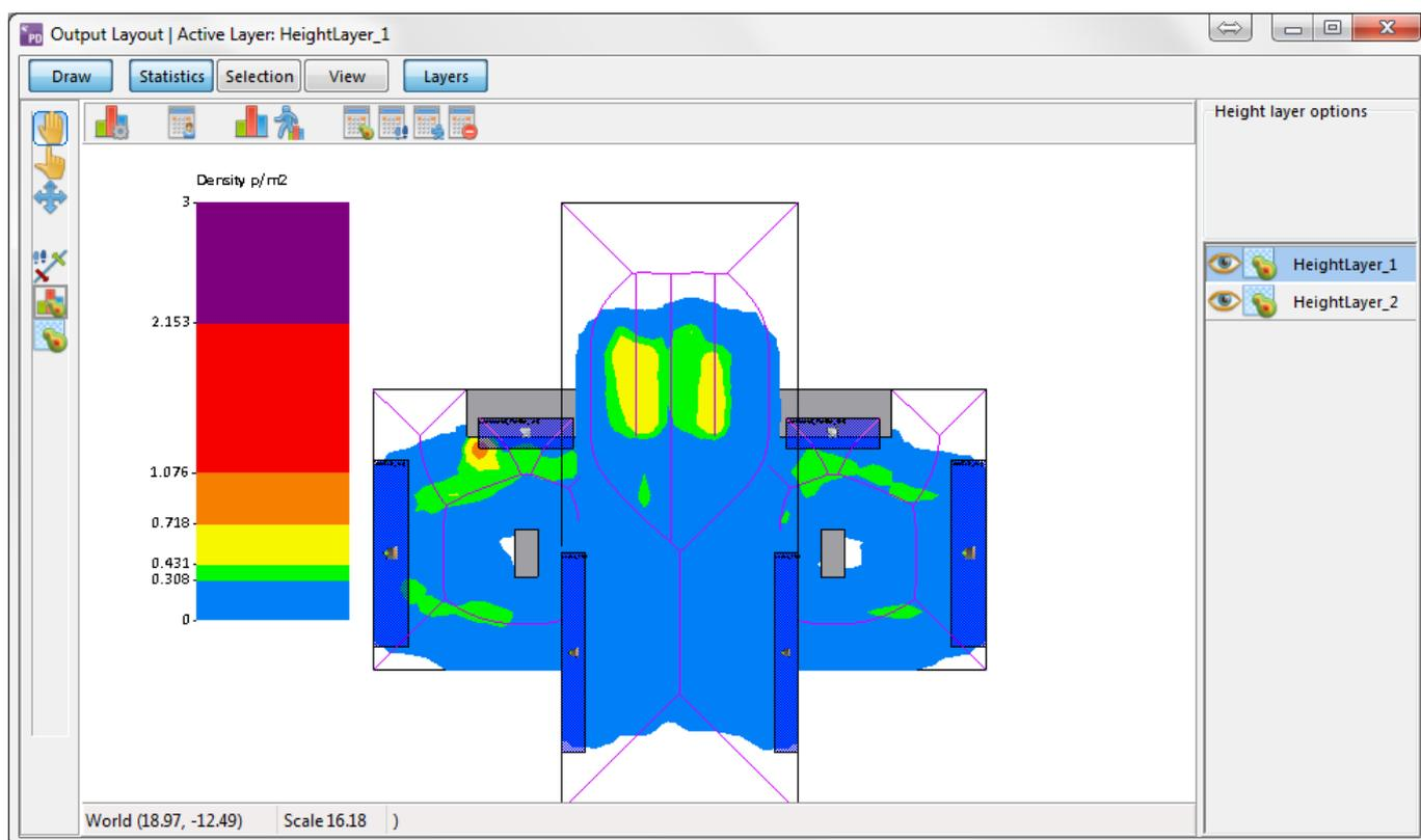
Figure 30: The 2D Output window showing the density map of HeightLayer\_2 of the tunnel7 model.
