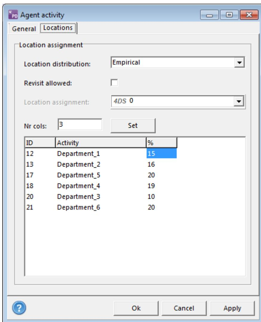
Figure 3: The Locations settings of the Shop activity. The location is assigned based on an Empirical distribution. In the table percentages for each location define the probability that an agent will visit this location when performing the shop activity.
