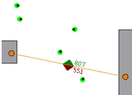
Figure 6: A flow counter showing the number of persons passing either way across the line.
