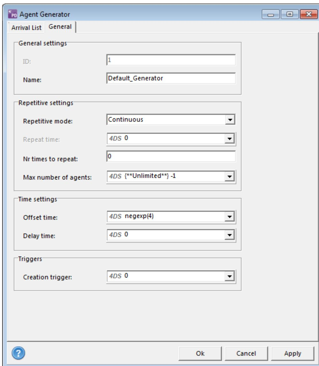
Figure 4: The General settings of the Agent generator configured as a random generator.
